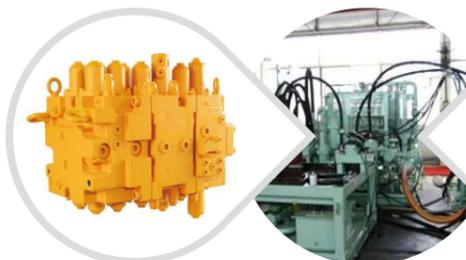
With pump-valve endurance test bed, the service life of main pump and main valve are tested and analyzed. In combination with research achievements of long-life parts of the customer, the service life of the pumps and the valves is improved by **1 time**.
