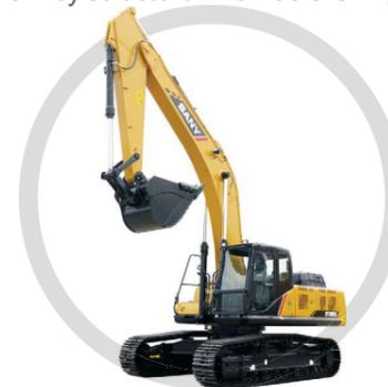
The boom adopts box-type structure with higher strength and is made of high-strength steel plates through advanced welding and molding process. The service life under mining conditions is **four times** of common boom.
