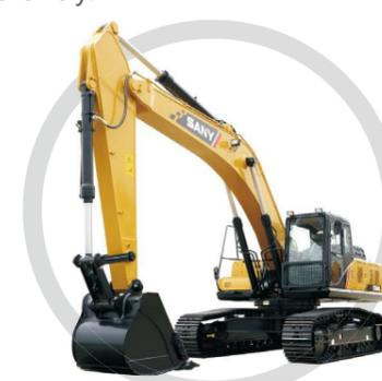
Bucket rod adopts bottom plate reinforcing bars and forging front support etc. As compared with competitor brands, the stress on main loading point is **30% lower**, and the service life is **30% higher** under mining conditions.
