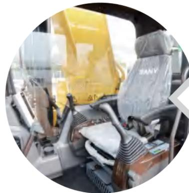
FOPS/ROPS cab is used. Through finite element modal analysis, steel structure and sealing performance of the cab are optimized; its strength is 5 times of general cab, the safety performance is extremely high and meanwhile the cab noise is reduced by 3-5dB, which makes the operation more comfortable.
