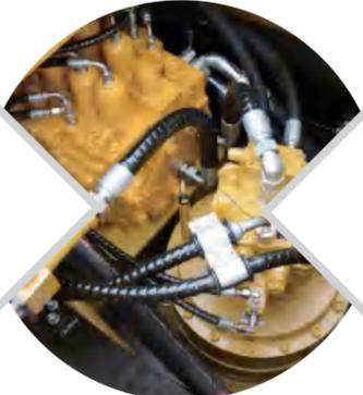
Kawasaki 32NA main valve is developed and designed according to customer requirements of SANY and has outstanding advantages including " high reliability, low pressure loss, high flow distribution efficiency and smooth compound control action" . It helps the customer create greater value.
