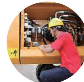
Replace diesel oil filter element
