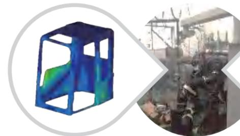
With vibration test bench and test bed, fuel tank and the cab has been tested by over hundreds of thousands of times on aspect of the vibration to improve the service life of the component by 50%.
