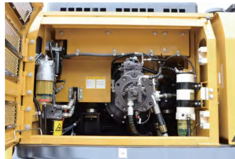
Large-capacity multi-stage filter system
