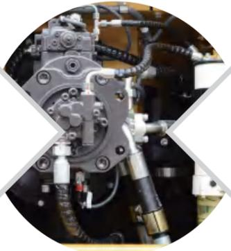
Kawasaki 160CC dual-ratio positive-flow main pump takes full advantage of the flow and realizes demand equal to supply. As compared with negative flow system, it reduces the loss of neutral-position return, and meanwhile response speed is higher and capacity loss is reduced
